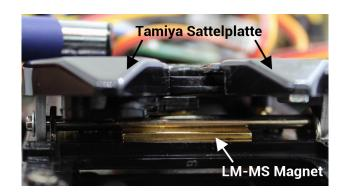
The king pin must be made of a material that transmits the magnetic field lines well, for example steel or iron. King bolts made of stainless steel or aluminum are not suitable here.
