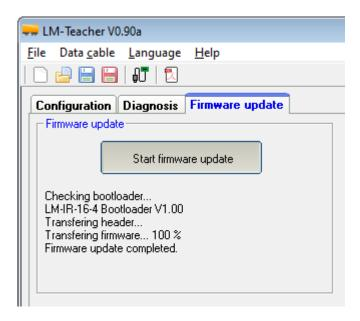
The right firmware for the light module is always integrated in the LM-Teacher. If there is an update for the LM-Teacher, a new firmware for the light module is always loaded.
