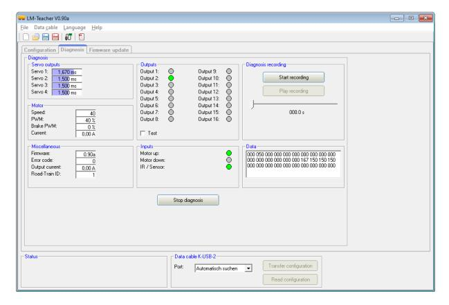
A diagnostic function is integrated in the LM-Teacher. This feature is very helpful to check the various functions of the light module. The data cable <a href="K-USB-2">K-USB-2</a> must be connected to X5/7 at the light module.
